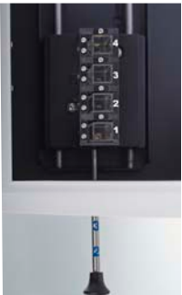
4-position cell holder 10x10 mm
