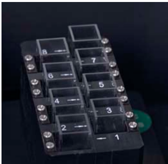
8-position auto cell changer - optionally
